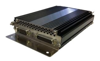
The Alto Acapella Series CA-003 is a TSO-C139a certified line level cabin audio selection controller with 4 stereo inputs and a PA mute feature. The unit provides 6 line outputs that can be configured to drive 3 stereo amplifiers or zones.
