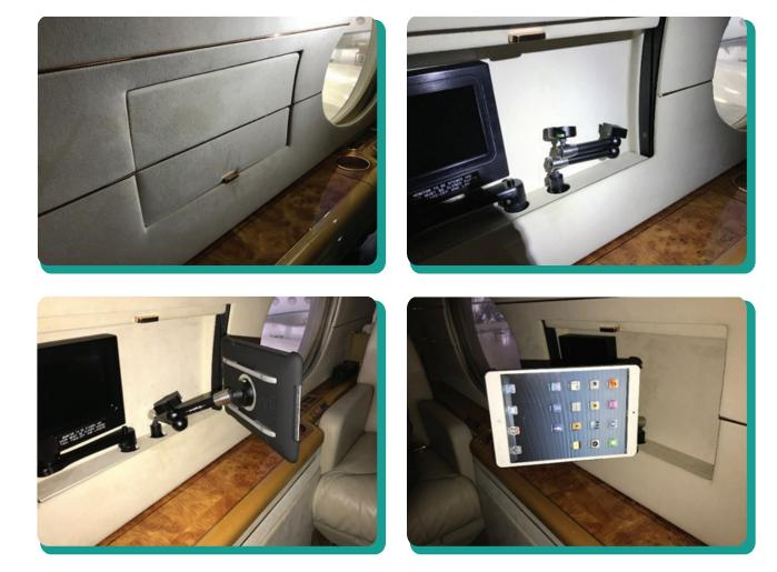
Here are some examples of the Articulating Plug-In Tablet Arm installed in a Gulfstream aircraft.
