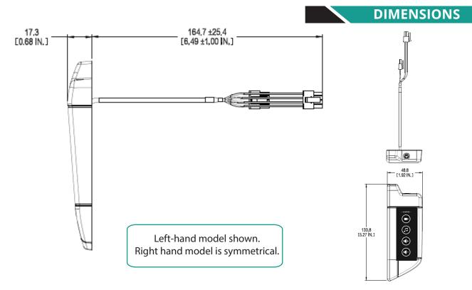
Note: Dimensions are for reference only. See DA (Delivered Assembly) drawing for exact dimensions
