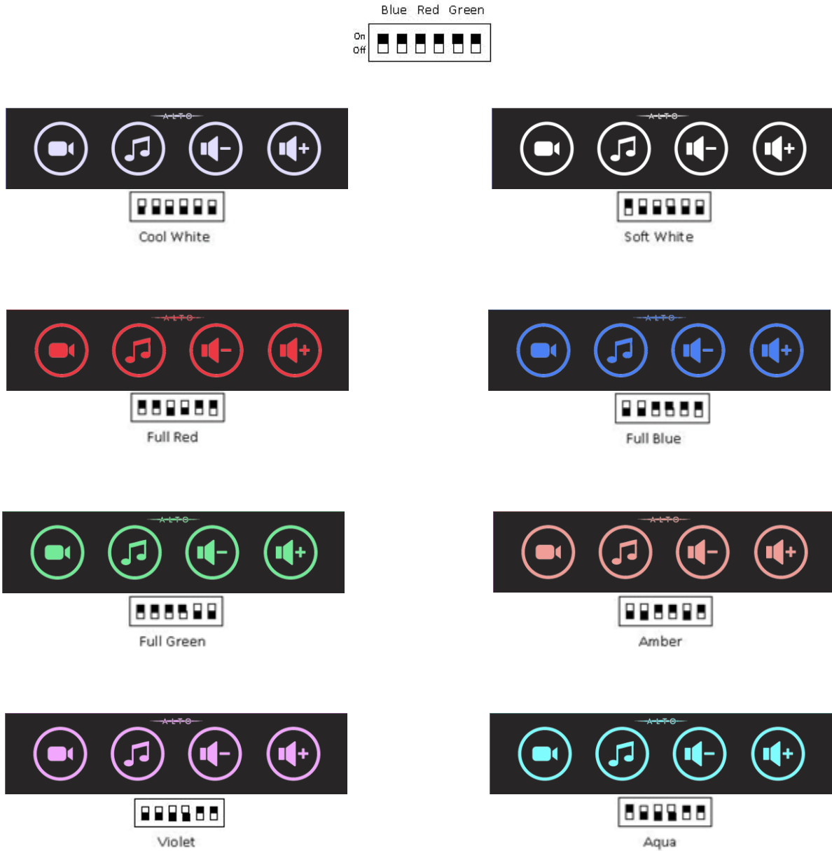
Figure 12: Example LED Color Select Diagram
