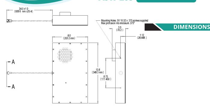
Note: Dimensions are for reference only. See DA (Delivered Assembly) drawing for exact dimensions. If the dimension, weight, and connector specifications of this product do not meet your requirements, ALTO can custom design a product for your application.
