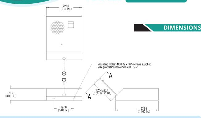
Note: Dimensions are for reference only. See DA (Delivered Assembly) drawing for exact dimensions. If the dimension, weight, and connector specifications of this product do not meet your requirements, ALTO can custom design a product for your application.
