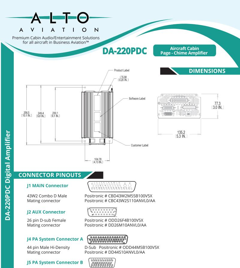
29 pin Male Std-DensityD-SubPositronic # MD29M5B100V5XMating connectorPositronic # RD29S10ANVL0/AA-1738.0
